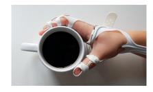
muscle movements in your forearm when you are getting ready to grasp an object, and applies the requested strength to your fingers via external tendons. The actuator of the tendons is strapped to your forearm and includes the motion sensors as well as the battery-driven power supply.
